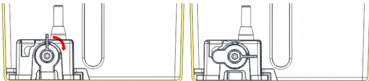
5. Slide the waterpump out of the bracket, see the schematic diagram here on the left.
