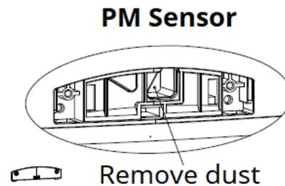
3. Clean the sensor lens with a cotton swab and water as indicated by the arrow. Then dry the lens with a clean cotton swab.
